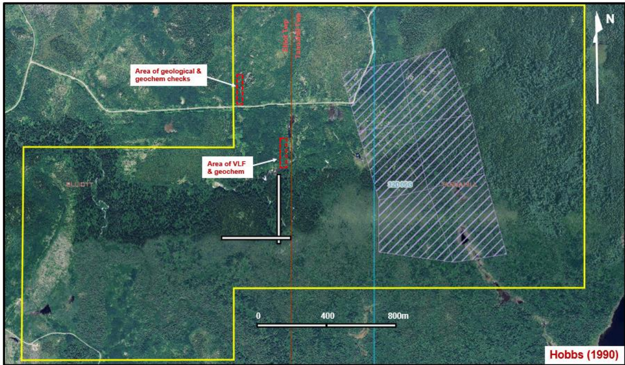
Figure 19: Location plan of the 1990 VLF-EM survey and geochemical test lines report by L. G Hobbs on the Bastarache property.
