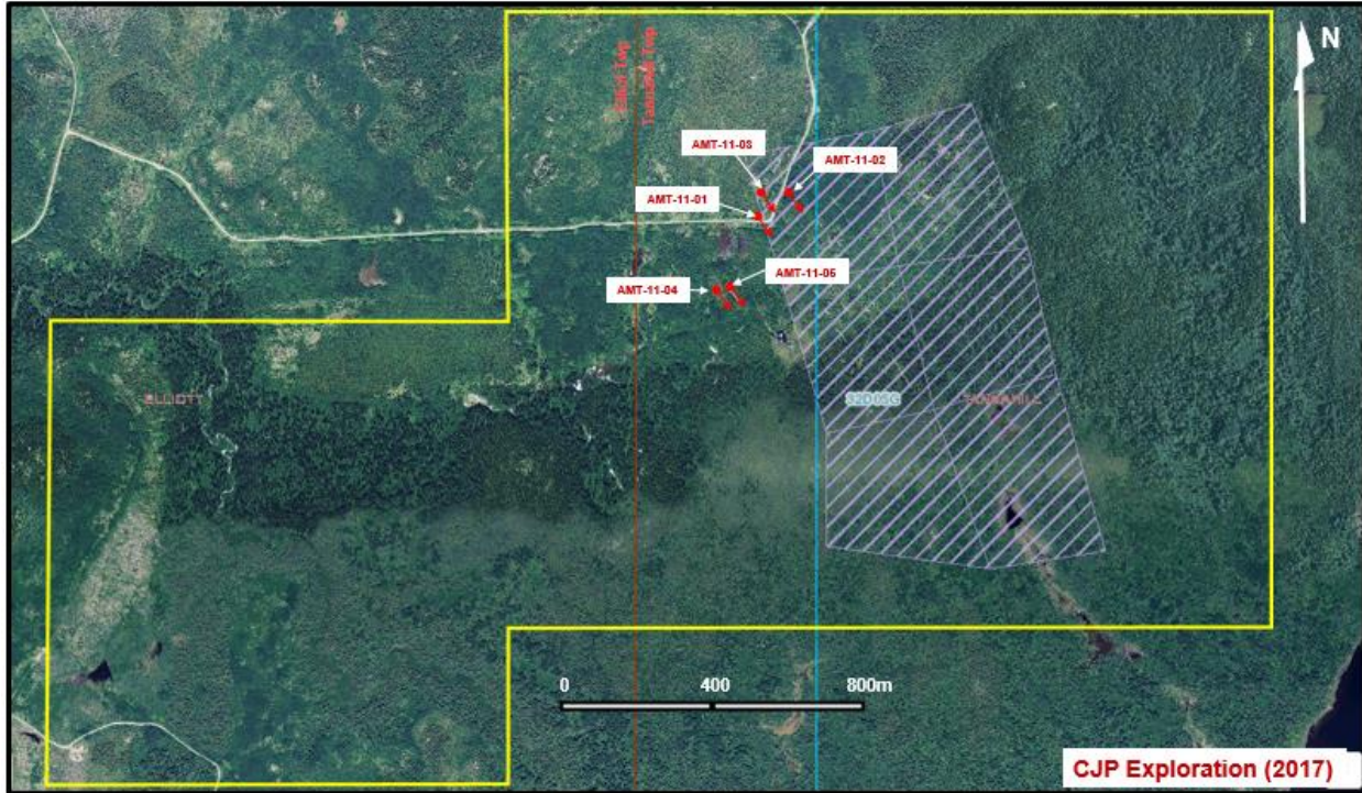
Figure 32: Location plan of the 2011 drill holes on the Abitibi Mining Corp property recovered and logged by C. J. Ploeger in 2017.
