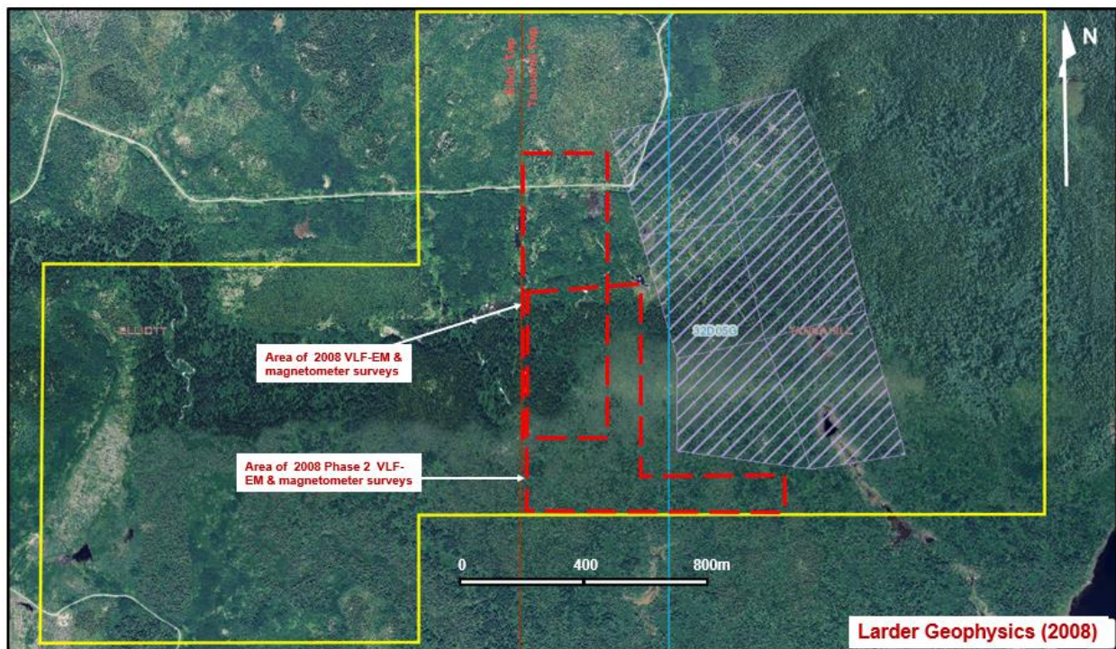
Figure 24: Location plan of the 2008 VLF-EM survey reports by Larder Geophysics on the Golden Chalice/ Abitibi Mining property.
