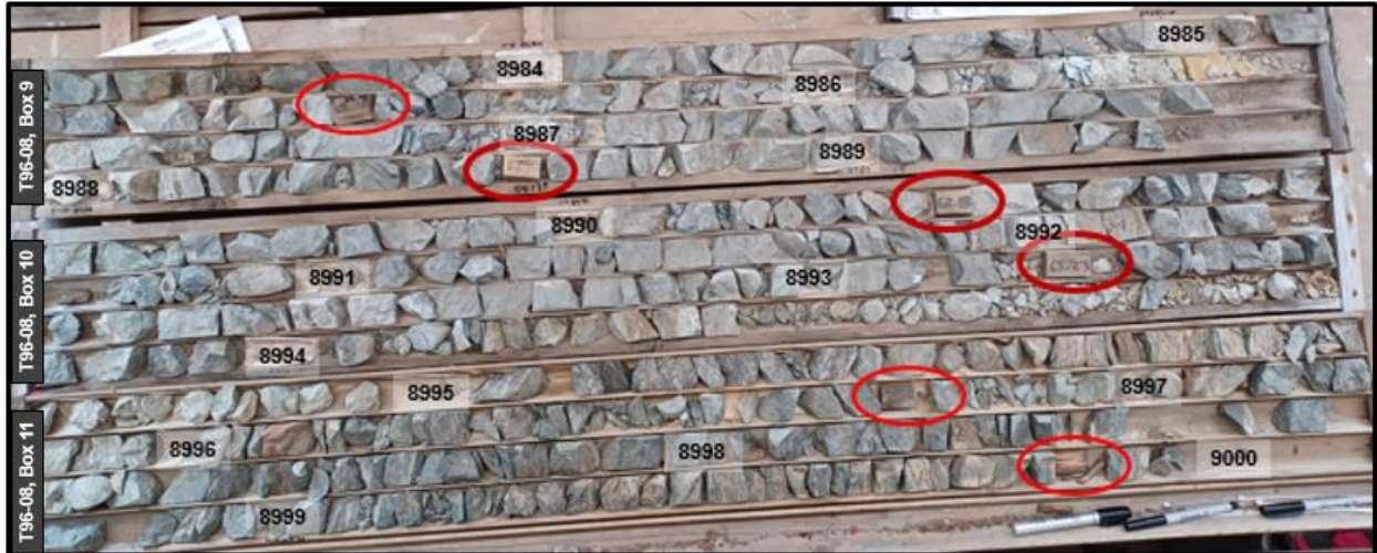
Figure 41: Hole T96-08: Consecutive footage blocks circled in the darker red contain the original markings from the drillers (194 ft= 59.13 m) and the metric conversion by the loggers (62.18m= 204 ft & 65.23 m= 214 ft) but the distance between the 194 ft (59.13 m) block in box 9 and the 204 ft (62.18 m) block in box 10 is only 5 feet (1.5 m). The original logging and sampling ignored this discrepancy and continued 1m sample intervals throughout.
